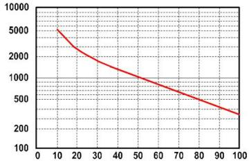
Battery life is directly related to how **deep** the battery is cycled each time. If a battery is discharged to 50% every day, it will last about twice as long as if it is cycled to 80% DOD. If cycled only 10% DOD, it will last about 5 times as long as one cycled to 50%. Obviously, there are some practical limitations on this - you don't usually want to have
